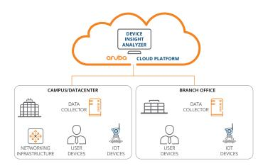
Attributes collected on the network are sent to ClearPass Device Insight Analyzer to accurately identify connected devices.
