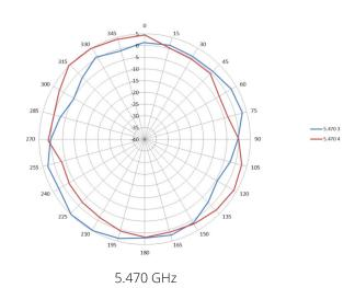
Elevation plane (side view, 0 degrees angle)
